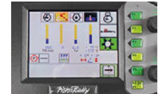
Integrated gradient sensors show the position of the blade and the vehicle in real-time.
