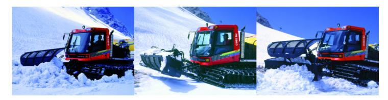
The perfect attachment for transporting snow over short to medium distances on the slope, lift or car park, e.g. for replenshing worn-out spots or for shunting and clearing work.
