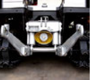
3-point rear power lift, Cat. 2, incl. cardan shaft 1 3/8 hexagonal profile (also as 3-point front power lift)
