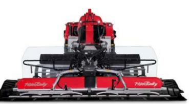
The hydraulically driven AlpinFlex Tiller Comfort is designed to provide ideal slope quality - even under extreme conditions. Innovative shape and arrangement of the tiller teeth. Built-in LED lighting. Memory function for saving and calling up all settings. Hydraulic locking of the tiller halves and hydraulically foldable side finishers. Equipped with a camera for maximum convenience.
