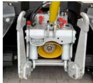
3-point rear power lift, Cat. 2, incl. universal drive shaft 1 3/8 hexagonal profile (also as 3-point front power lift)
