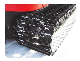
The X track cleat combines a steel core with a high quality vulcanized rubber encasement. The rubber encasement has a herring bone structure that gives the cleat excellent grip.
