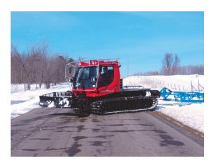
The X track provides traction when pulling snowmobile trail grooming drags in hard, icy snow conditions yet will not damage pavement when crossing roadways.
