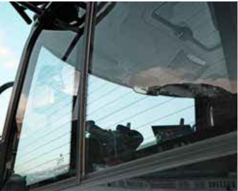
Dual sliding side windows, heated in any position, for optimum lateral visibility.
