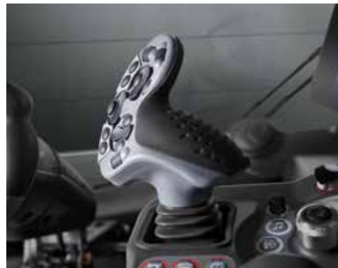
Joystick with ergonomic and proportional control for intuitive working.
