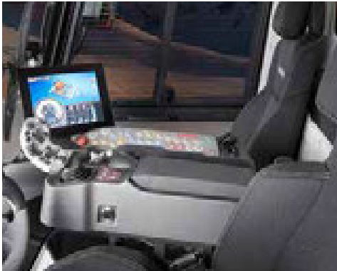
Optimized control even on uneven terrain thanks to the control unit integrated in the seat.
