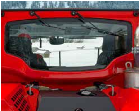
Larger and heated rear window for optimum visibility to the rear as well.
