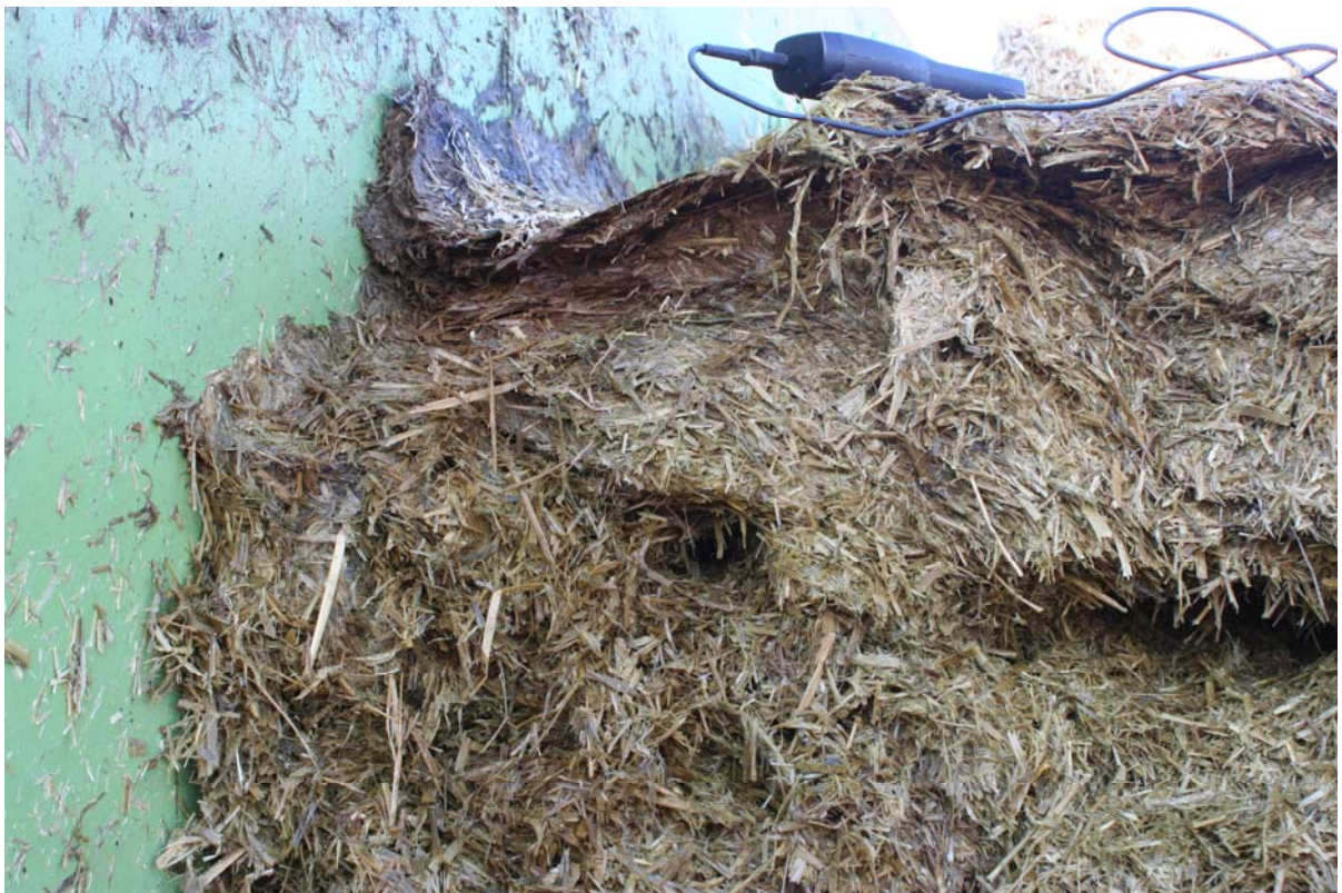
Figure 7: Temperature measurements in the bore holes
