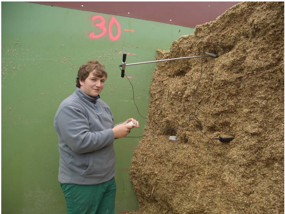
Figure 2: Temperature measurements in the bore holes
