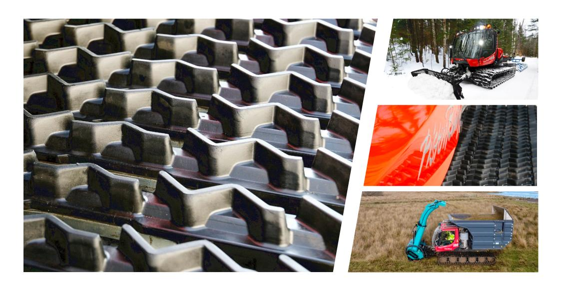
The X-Track chain grouser combines a alu core with high-quality vulcanised rubber cladding. The cladding has a herring bone structure that gives the chain excellent grip.
